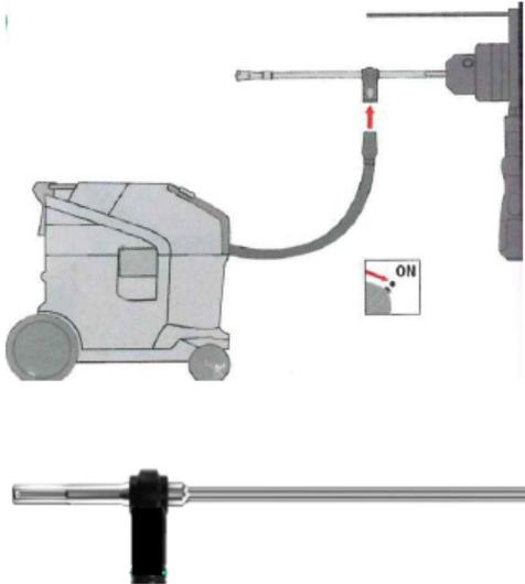
Switch-on the vacuum cleaner before to drill
